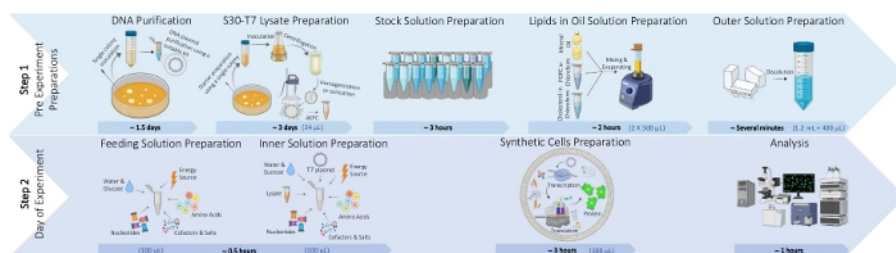
Figure 1: An illustration of the process for typical synthetic cells preparation protocol. The process is divided into two steps. Step 1: Pre-experiment preparations including DNA plasmid purification, S30-T7 lysate preparation, stock solutions preparation required for the inner and feeding solutions, lipids-in-oil solution preparation and outer solution preparation. Step 2: Synthetic cell formation that includes feeding and inner solutions preparation, synthetic cells preparation and analysis. An example of the required volume of each ingredient for preparing 100 µL of synthetic cells solution is presented in blue in brackets. Please click here to view a larger version of this figure.
